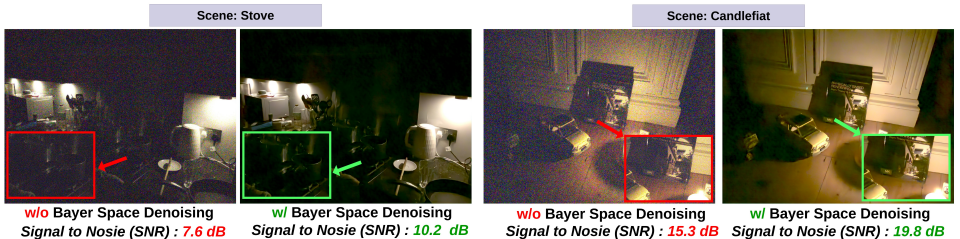
Figure 3: Importance of bayer space denoising using PMRID: Denoised raw images successfully retrieve scene information from noisy low illumination and saturated bright regions in the raw image space due to a lowered photon shot noise level.
